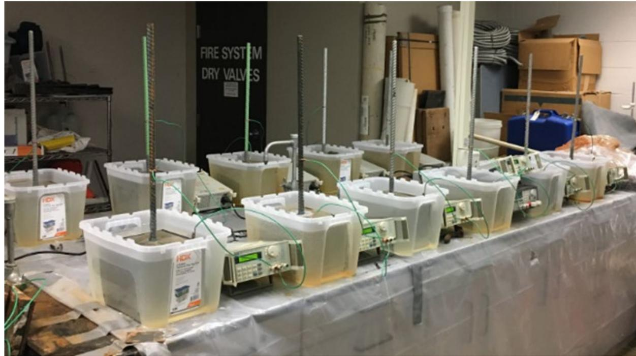
Accelerated Corrosion Test Set-up
